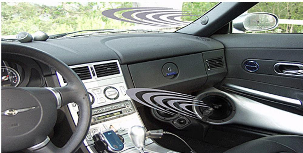
couple strongly to the mid/woofer and to be rotationally placed to time align the woofer dome and the Tweeter. This means there is an area defined by points, which are equidistant to the apex of the cone and the Tweeter diaphragm. Additionally the Tweeter, which itself is angled, may be directed during mounting. Finally one ideal mounting and listening position exists to provide the best of both.
